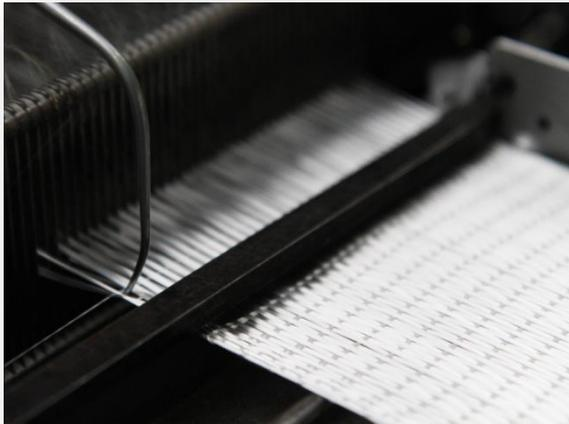
Eurocarbon is a producer of both woven and unidirectional tapes in several different styles and reinforcement materials. Tapes provide reinforcement in the 0 and 90 degrees direction.
